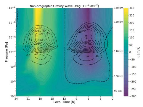
Fig. 17. Local time-pressure distribution of the GW zonal drag (contours) integrated over all latitudes ( $\theta$ ) and normalized by  $\cos(\theta)$  to account for conservation of angular momentum. Zonal winds (colour) at equator regions (10°S-10°N) are also shown. Solid line indicates acceleration, dotted line deceleration. Positive zonal wind values are westward and negative zonal wind values are eastward. Dashed-line indicates the region where the zonal wind converges to zero.
