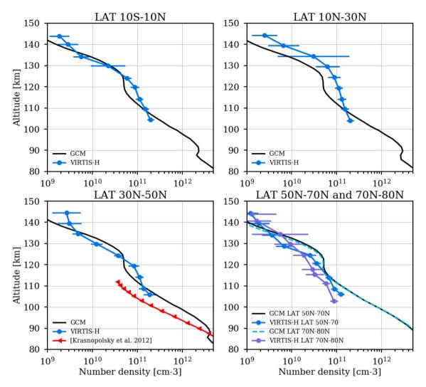
Fig. 7. CO density retrieved by VIRTIS/VEx during daytime (LT 10 h–14 h) after Gilli et al. (2015) together with IPSL-VGCM averaged profiles binned at similar latitude and local time, as indicated in the panels. In addition, semi-empirical CO profile from Krasnopolsky (2012) representative of mean conditions is shown for comparison with mid-latitude (30°N-50°N) daytime averaged profiles.
