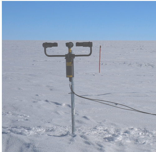
Figure 4.1: Initial location of the disdrometer : it was then moved to the top of a shelter [D. Six]
