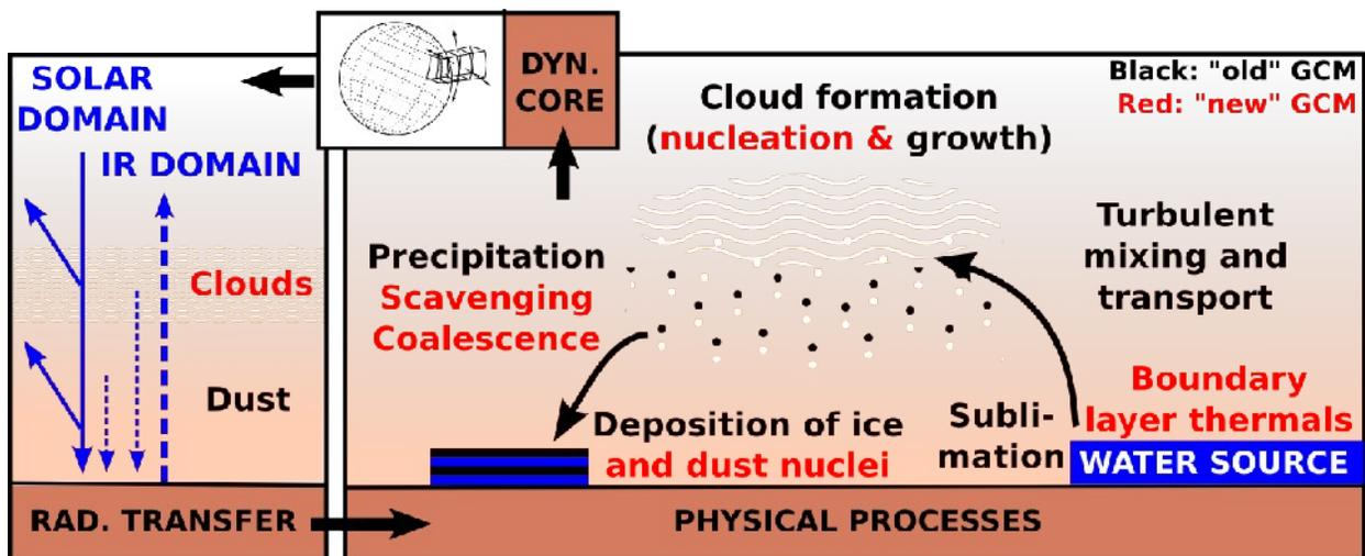
Figure 1: Diagram showing the main components of the LMD/GCM (the dynamical core, the radiative transfer code and the physical processes) as well as the new physical processes (in red) that have been recently implemented in the model.
