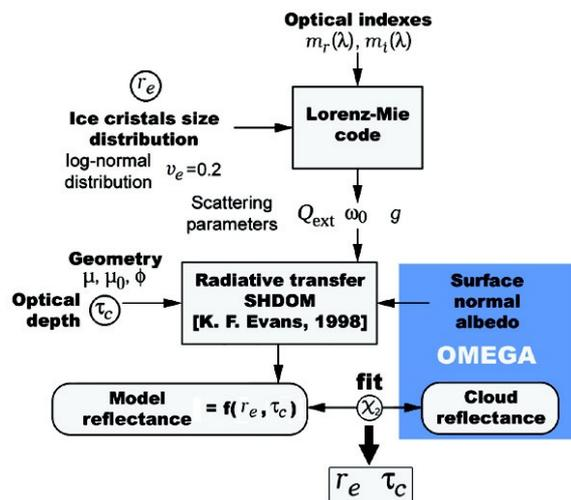
**Figure 1.** Schematic drawing of the water-ice crystals size  $r_e$  and cloud optical depth  $\tau_c$  retrieval method.
