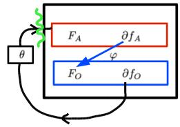
Open loop: system made insensitive to  $\theta$  by setting  $\vec{F}_A = 0$ . Equation reads  $\delta\theta = \delta\theta_{ins}^*$ .
