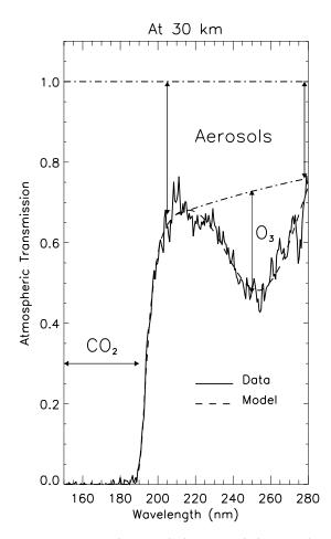
**Figure 45.** Spectral transmission recorded at 30 km of altitude during polar night (one single 1 s measurement). The ozone absorption trough is well seen, superimposed to the dust continuum above 200 nm of wavelength. Below 190 nm, there is a total absorption by  $CO_2$ .
