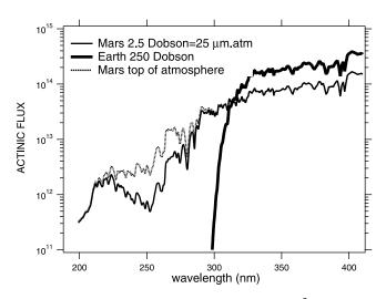
**Figure 42.** Solar flux in units of photons/(cm<sup>2</sup> s nm) for various cases. Thick solid line: Earth's case with a vertical column of 250 Dobson, SZA =  $60^{\circ}$ . Solid line: Mars case with 2.5 dobson = 25  $\mu$ m-atm, the maximum quantity that was found with SPICAM on the day side. Dotted line: at top of Mars atmosphere. This illustrates that ozone on Mars is insufficient to offer a proper protection from solar UV, while on Earth the solar flux is essentially 0 below 300 nm.
