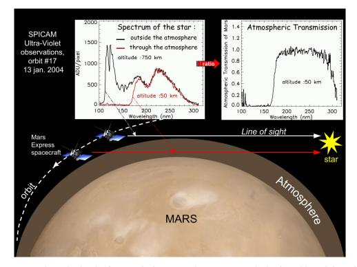
**Figure 30.** Schematic sketch of an occultation. From the two spectra obtained outside and through the atmosphere, an atmospheric transmission can be derived. Displayed spectra come from the very first stellar occultation made by SPICAM at the beginning of the mission, which is also the very first made by any instrument orbiting around Mars. Shortward of 180 nm, the signal is completely attenuated by CO<sub>2</sub>.
