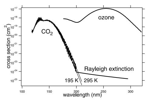
**Figure 29.** Absorption cross sections of  $CO_2$  and ozone, with Rayleigh extinction of  $CO_2$  in the UV spectral range of SPICAM. The  $CO_2$  cross sections are shown for two temperatures. At 200 nm, it is larger for 295 than 195 K. Aerosols/dust would add to the absorption.
