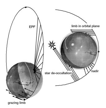
**Figure 6.** Sketch of various modes of observation of SPICAM. In all cases, the black line indicates the LOS of SPICAM to the target. Except for the usual nadir orientation and the special case of EPF (Emission Phase Function), the spacecraft is drifting along the orbit, keeping a constant celestial orientation, which allows us to scan across the target (limb) or to perform an occultation of star or Sun.
