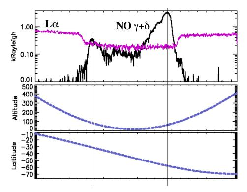
**Figure 25.** (top) Integrated intensity (wide slit band corresponding to Figure 23, top) of both the L $\alpha$  emission and the whole NO band from 190–270 nm, as a function of time. (center) Altitude of the tangent point MNP. The NO emission displays two peaks, each time the LOS crosses the 70 km altitude. The second peak is brighter by a factor ~10 and is at high southern latitude. (bottom) Latitude of the tangent point MNP (adapted from *Bertaux et al.* [2005a]).
