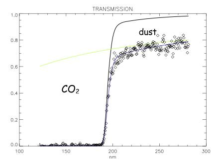
**Figure 34.** Same as Figure 33, but lower in the atmosphere. The green curve is the absorption attributed to aerosols necessary to fit the data, in addition to  $CO_2$  absorption and Rayleigh extinction. In this particular case, there is no ozone.
