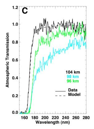
**Figure 39.** The measured spectral transmission recorded at three altitudes during a stellar occultation is fitted by a simple spectral extinction law, defined by the Angström coefficient. During this occultation, a high-altitude cloud of  $CO_2$  ice particles was detected (see section 7.4.4). The transmission is smaller at 98 km than at 96 km, revealing the presence of the absorbing layer. The spectral slope is also different at the altitude of the cloud.
