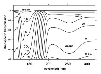
**Figure 32.** Synthetic spectra of Mars atmosphere transmission in occultation for various grazing altitudes. Dust is taken into account here, most visible as a continuous and sloppy absorption above 210 nm, and ozone is present as an absorption trough clearly visible at 30 and 40 km of tangential height. The curve at 30 km may be compared to the actual measurements of Figure 45.
