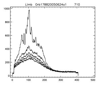
**Figure 15b.** During the one second exposure corresponding to the geometry of Figure 15a, the 5 spectra recorded at 5 points of the narrow slit are represented. The nearest point to the limb sees a normal solar spectrum (scattered by dust at the limb), while the others, further away, see only stray light generated through the large portion of the slit. A series of such measurements allowed us to characterize the stray light and correct for it.
