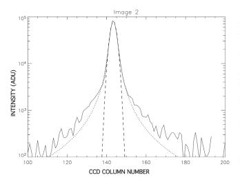
**Figure 12.** Solid line: distribution of light along the column axis of the CCD (perpendicular to the dispersion direction) of a stellar image taken in the Imaging mode, during the cruise to Mars, displayed in Figure 8. All wavelengths are summed together. The dashed line is a Gaussian fitted to the central part, while the dotted line is a Lorentz profile fitted also to the external part.
