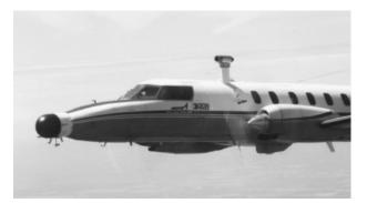
FIG. 1. Photograph of the AUSAT mounted above the fuselage of the Merlin IV in 1996.
